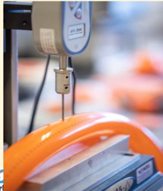
Automated pressure monitoring of bike tubes (Copyright: Tubolito GmbH)
