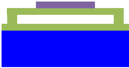
Silicon nitride plate realized using the sacrificial release process (Vertical dimensions and material properties not easy to control)
