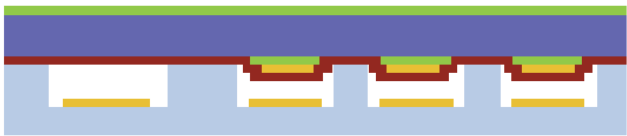
After anodic bonding and handle wafer removal
