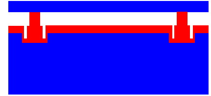
Extended dielectric posts realized by LOCOS process improve reliability and decrease the parasitic capacitance (limits minimum lateral dimensions)
