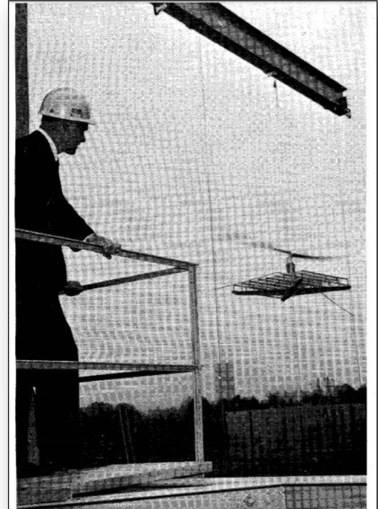
Fig. 5. Microwave-powered helicopter in flight 60 ft above a transmitting antenna. The helicopter was demonstrated to media in October 1964. A 10-h sustained flight was achieved in November of that same year.
