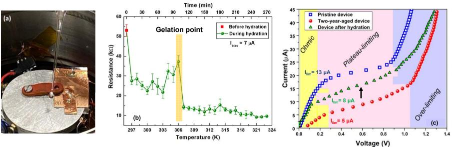
The regeneration process initiates at the gelation point (~306 K), resulting in a more conductive nanocomposite.
