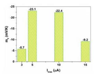
Voltage temperature sensitivity  $m_V$  is current-dependent
