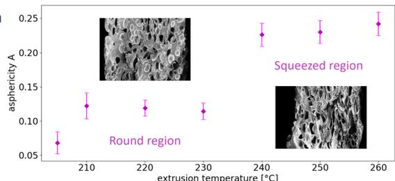
**Figure 4 - Average asphericity of sample cells printed at different extrusion temperatures**
