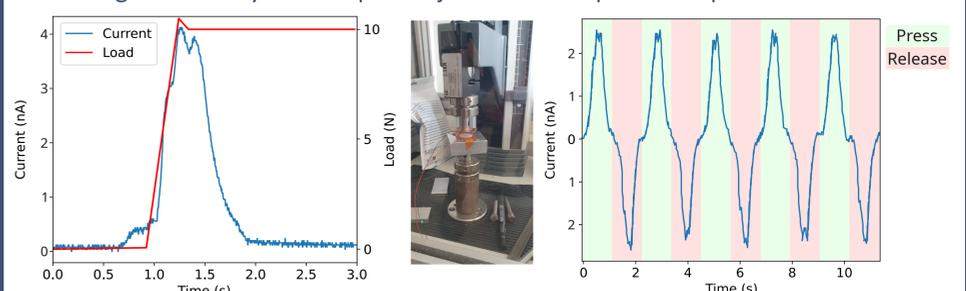
**Figure 7 - Short-circuit current, the experimental setup and a series of compression and release cycles**
