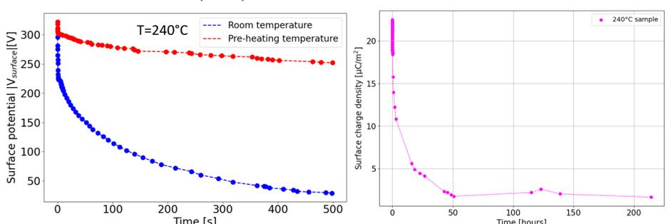
**Figure 6 - Temporal decay of surface potential values and surface charge density of a 240°C-printed sample**
