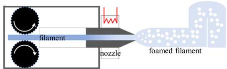
Foam-controlled 3D-printing by varying extrusion temperature and flow rate
