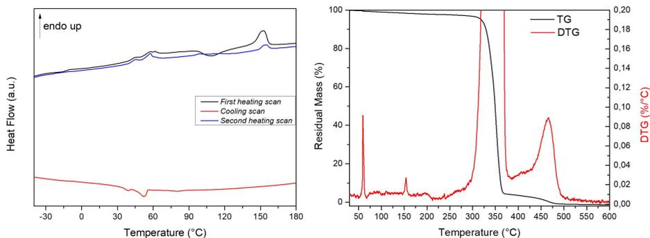
**Figure 1 - Differential scanning calorimetry (DSC) and thermogravimetric analysis (TGA) of the filament** Plots indicate the presence of a low-melting polymeric blowing agent at 45.3°C and the thermal degradation of the microspheres is responsible for the material foaming
