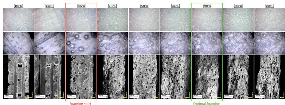
**Figure 3 - Optical images of 3D-printed LW-PLA samples and relative SEM images of their cross sections**
