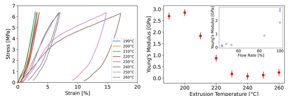
**Figure 5 - Compressive stress as a function of percentage compressive strain and measured Young's modulus as a function of extrusion temperature and flow rate (inset)**
