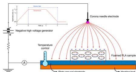
Simultaneous negative corona charging and thermal treatment of samples
