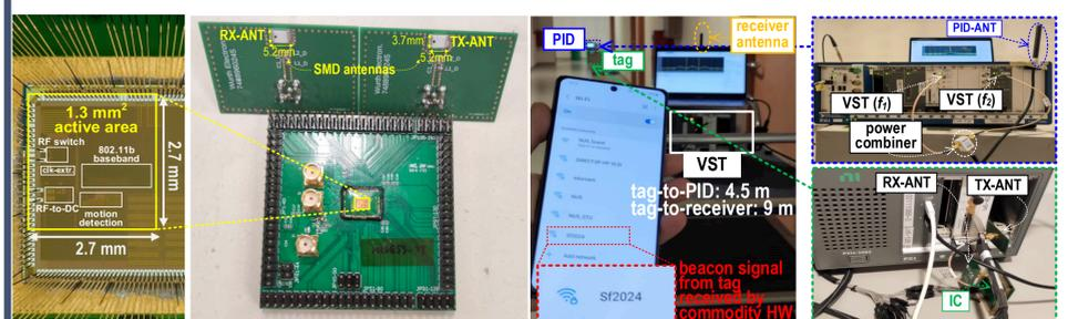
Figure 2 – IC microphotograph (TSMC 180nm), custom PCB, measurement setup
